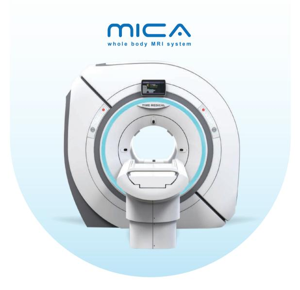
The 1.5T MICA Whole Body MRI System comes with zero boil-off superconducting magnet which does not require regular refill of liquid helium. The wide range of clinical applications allows professionals to perform all types of scans to patients from routine pulse sequences to advanced clinical diagnosis. The integration of Prodiva platform allows simple workflow with consistent great image quality resulting in higher patient throughput and productivity.
